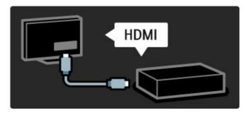
The HDMI connection offers the best picture and sound quality and, if your device has **EasyLink** (HDMI-CEC), the TV can add the device in the Home menu automatically.
